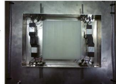
Figure 9. The design of the luminosity monitor features four low noise photo multiplier tubes in sets of two. We measure counts from coincidences of each pair of PMTs, and all four together. A block of polyethylene provides a filter for protons below 500 MeV/c and pions below 150 MeV/c.
