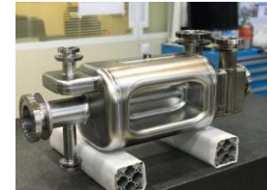
RF dipole (RFD) cavity
