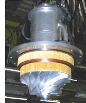
Impeller of an LHC cold compressor stage
