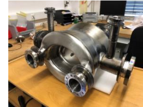
Double Quarter Wave (DQW) RF cavity
