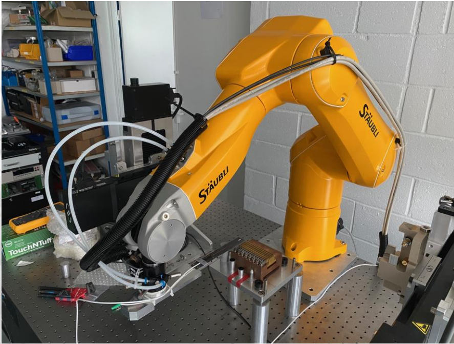
Figure 32 : Robotic arm scanning the supermodule with a 3D Hall probe
