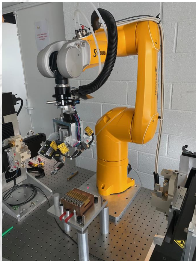
Figure 30 : Robotic arm adjusting a Supermodule
