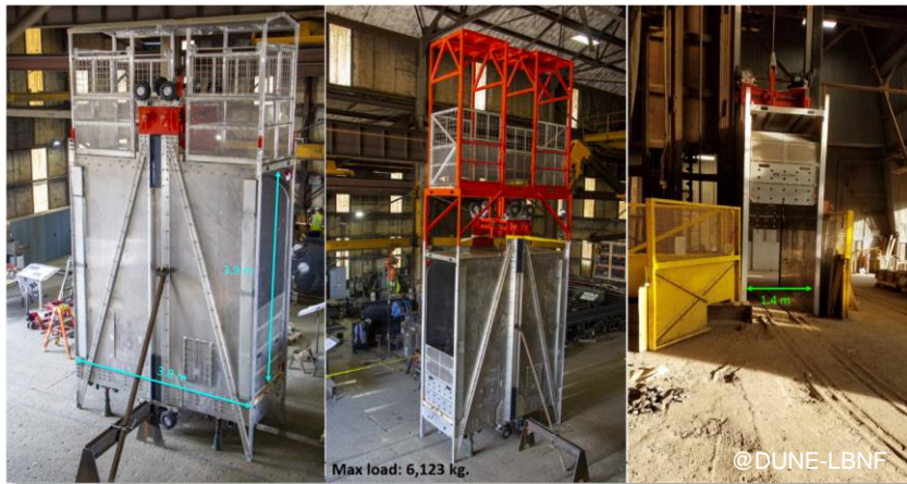
Argon condensers: approx. 1.3 m 3 LN 2 , 1.8 m 3 LAR Sizes: 2.5 to 5 m height; 1.2 m diameter
