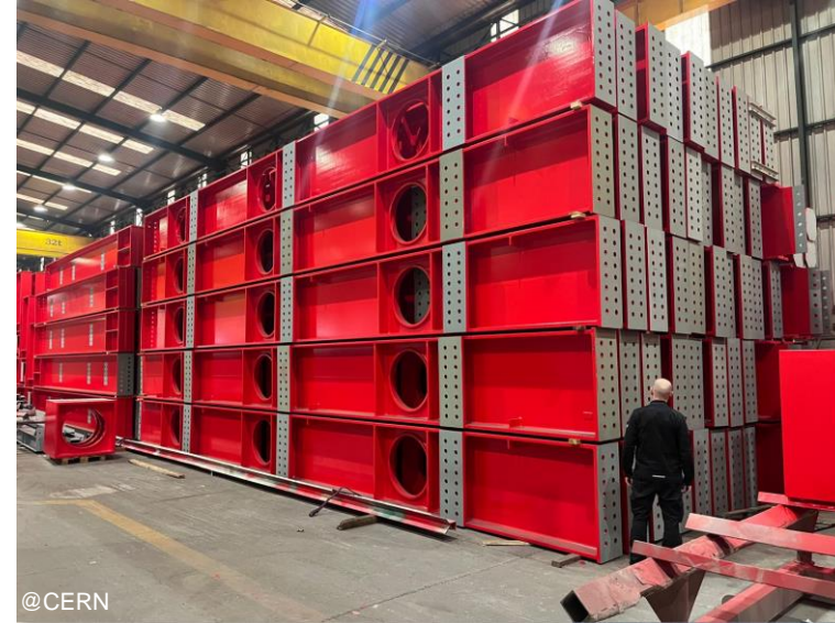
The metal structure of the first cryostat at Horta Coslada (Spain)
