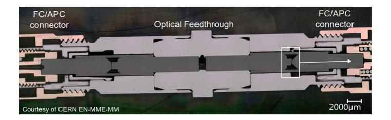
Continuous optical fibre from room temperature/atmospheric pressure to cryogenics/vacuum
