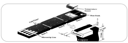
Design, manufacture and assembly of a new type of thermometric block and support for a cryogenic thermometer measurement chain. The thermometer has been tested, produced in series and validated to function accurately under adverse environmental conditions.
