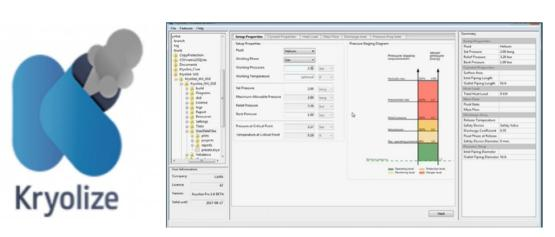
Kryolize is a software tool for sizing the minimum discharge area of a safety protection device, against overpressure. Based on international (ISO), European (EN) and American (API) standards, Kryolize allows for the calculation and sizing of safety valves for cryogenic systems.
