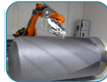
CFRP tank prototype production - CASA Espacio (2014)
