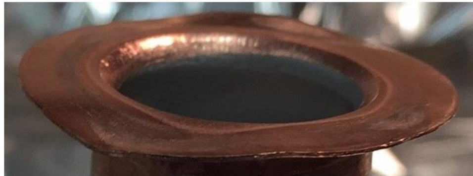
Figure 7.10 Flange deformation due to high temperature (650 °C). The copper becomes softer and lose his mechanical properties. A deformed flange is a very probable source of vacuum leaks, avoiding the possibility of the rf test.
