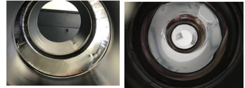
The inner surface of a large grain cavity before and after mechanical polishing.
