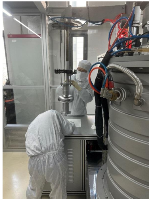
The top flange of the cavity was covered with niobium foil.
