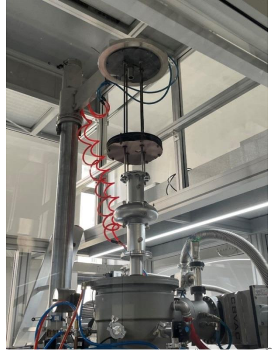
The top flange of the cavity was covered with niobium foil.
