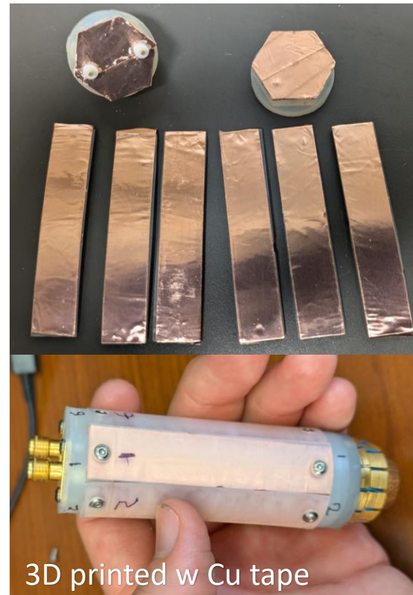
FSU 3D printed Cu tape hexagonal cavity
