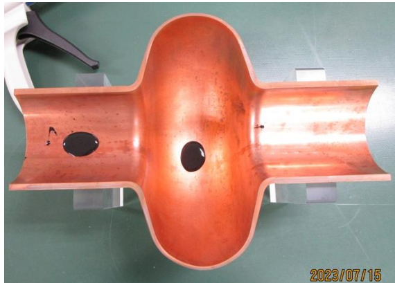
Plastic replica is used for roughness measurement
