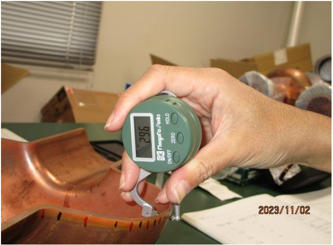
Thickness was measured by caliper
