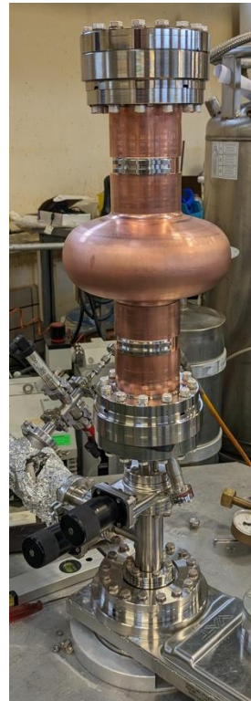
Cavity on the HPR setup
