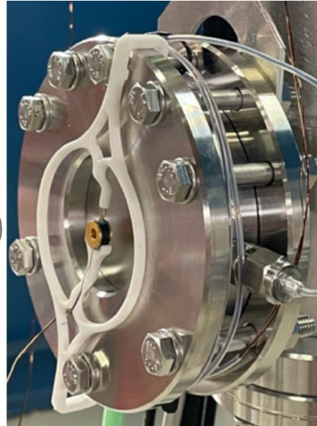
T-sensor inside & outside Manganin heating wire inside
