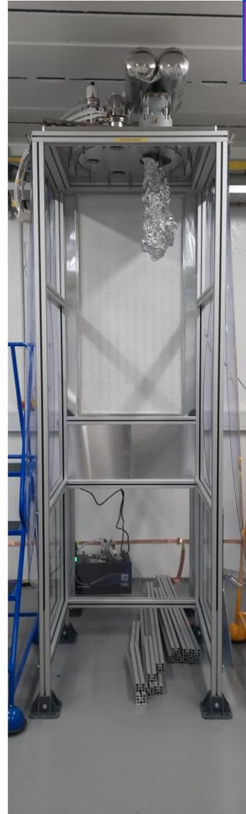
Magnetic shields, Vacuum chamber and thermal radiation screen
