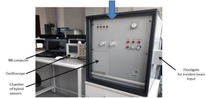
Particle identification, fluxmetry and dosimetry instrument „VUTEG-7“ (front view)
