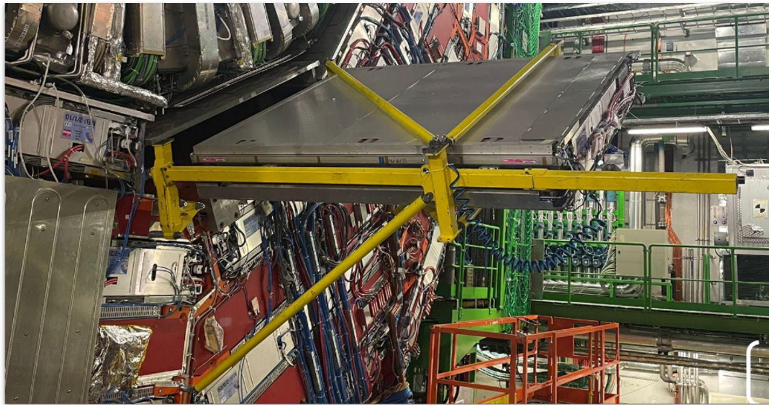
Two full RPC chambers extracted using a new procedure including replacement of the gas pipes
