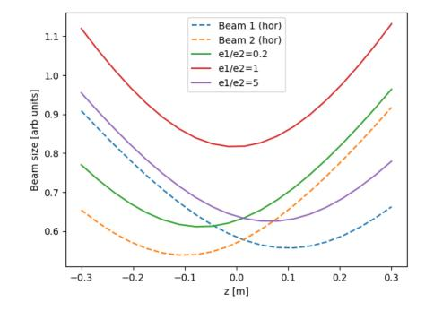
In this example the waist is shifted by 0.1 m for beam 1 and by -0.1 m for beam 2. For scans with equal emittances in the two beams the minimum is in the centre, but not when the emittances are different.
