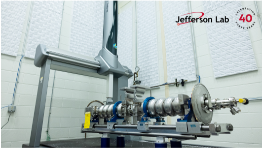
Figure 10: RF accelerator cavity
