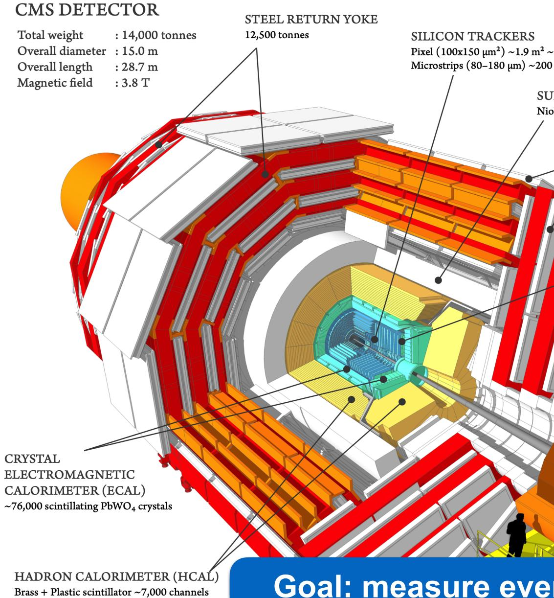
ELECTROMAGNETIC CALORIMETER (ECAL) ~76,000 scintillating PbWO<sub>4</sub> crystals
