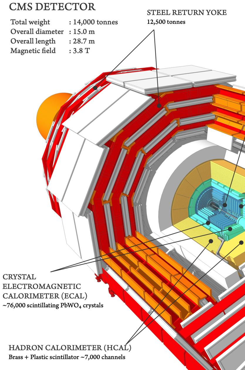
SILICON TRACKERS Pixel (100x150  $\mu m^2$ ) ~1.9 m² ~124M channels Microstrips (80–180  $\mu$ m) ~200 m<sup>2</sup> ~9.6M channels
