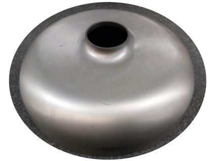
Nb half cell after 1 st calibration. Fabrication is in process at vendor
