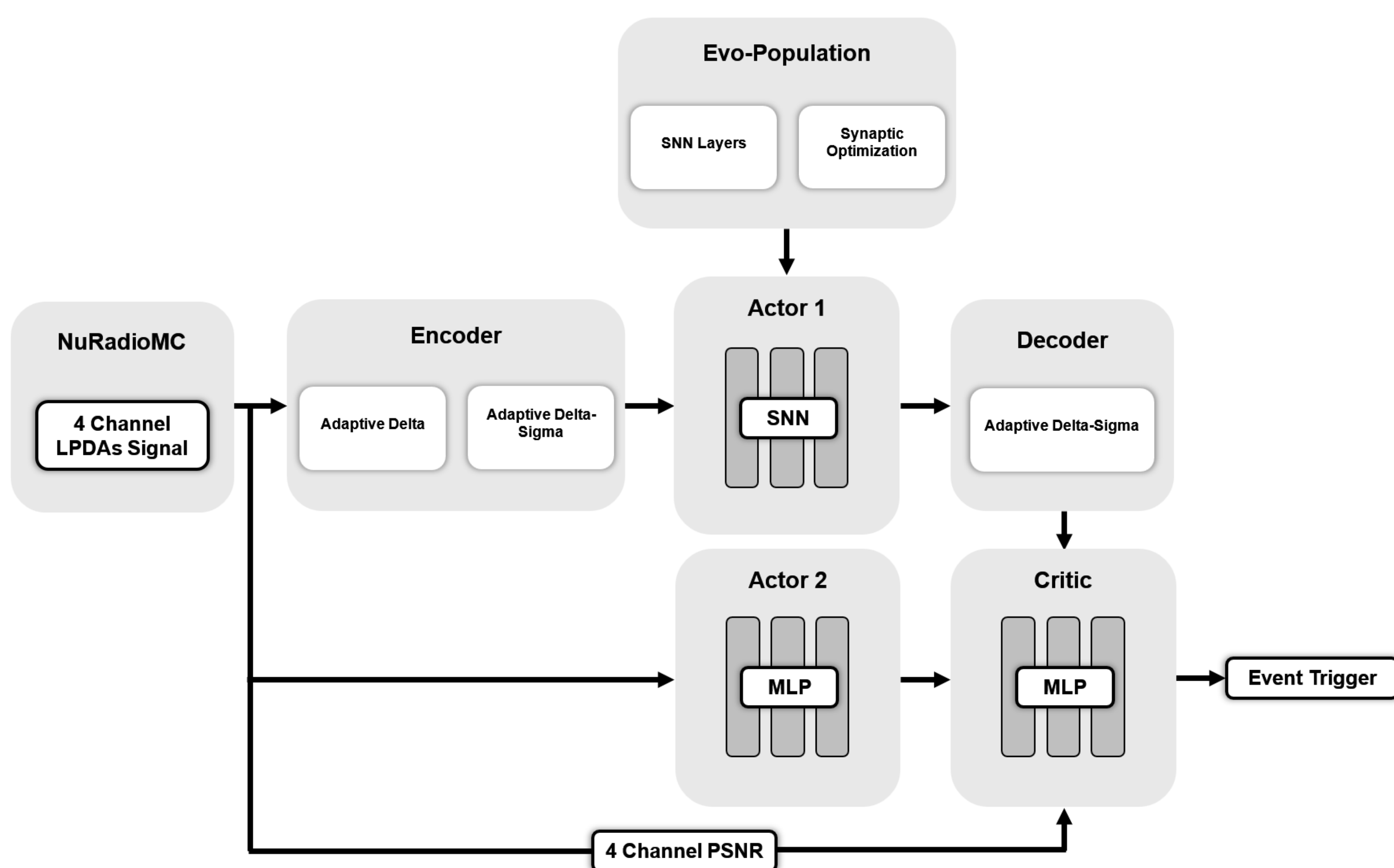
Fig. 3: The overall view of Evo-SAN pipeline which is composed of two actor networks, a single critic network for action selection based on privileged observation, and an evolutionary population generation based on Spike Neural Network (SNN).
