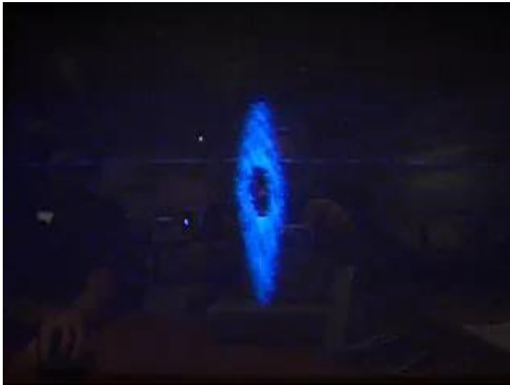
Synchrotron Radiation Monitor showing the transverse beam shape
