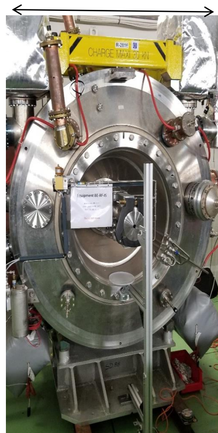
Accelerating Cavity, freq = 80 MHz (CERN PS) All pictures © CERN
