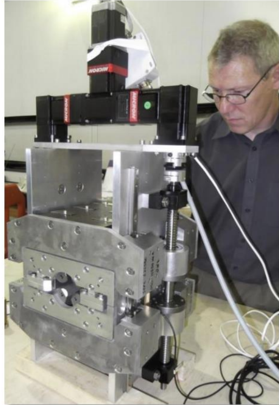
Tunable quadrupole for CLIC drive beam (B. Sheperd STFC)
