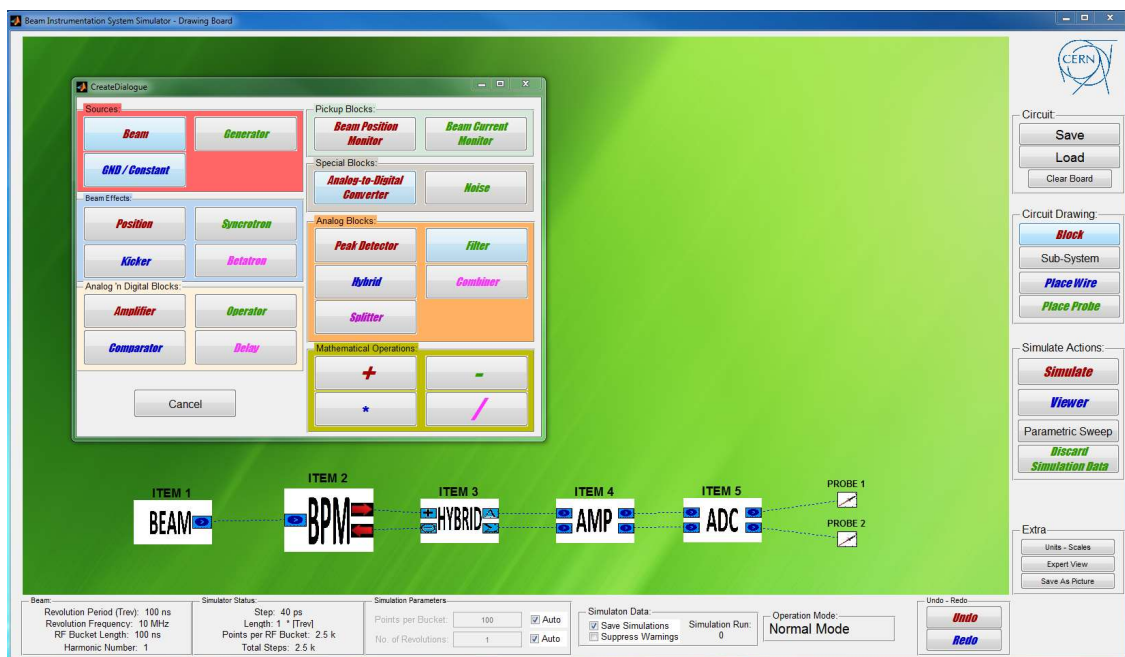
Fig. 1: Workspace with circuit drawing Block open
