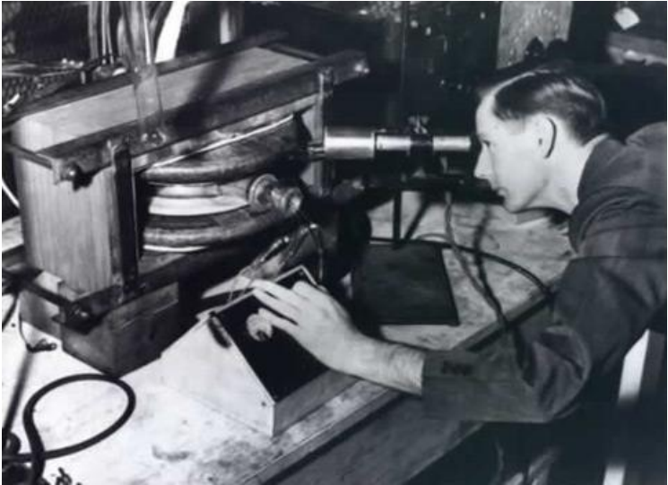
Donald Kerst with the first betatron, invented at the University of Illinois in 1940
