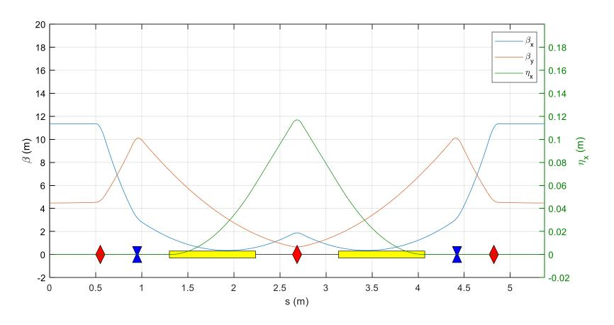
DBA cells have a dispersion function that is mirror-symmetric about the centre with zero dispersion away from the dipole pairs.
