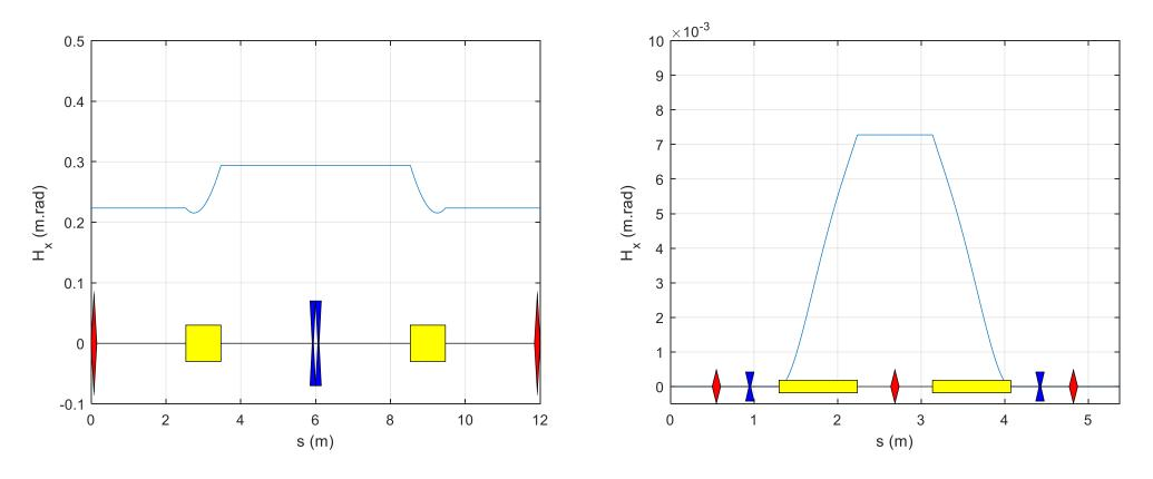
The function  $\mathcal{H}_{\chi}$  is much smaller in the DBA lattice (right) than in the FODO lattice (left).
