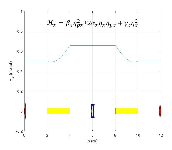
As a first attempt at reducing the natural emittance, we can try reducing the function  $\mathcal{H}_{x}$  in the dipoles by designing a lattice that has zero dispersion at either ends of a dipole pair.
