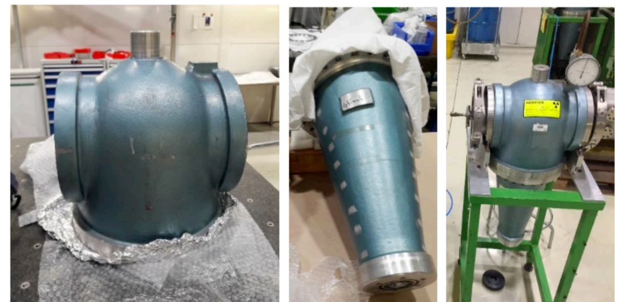
Fig. 4-31: New Cerenkov counter. Left: body; centre: conical part; right: complete assembly.
