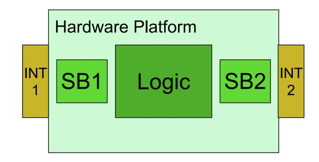
**Example**: Hardware platform ready to be tested, but missing input source SB1 can be used in playback mode to emulate data from interface 1
