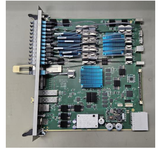
MUCTPI board with two Virtex UltraScale+ XCVU9P FPGAs and one Kintex UltraScale XCKU095 FPGA
