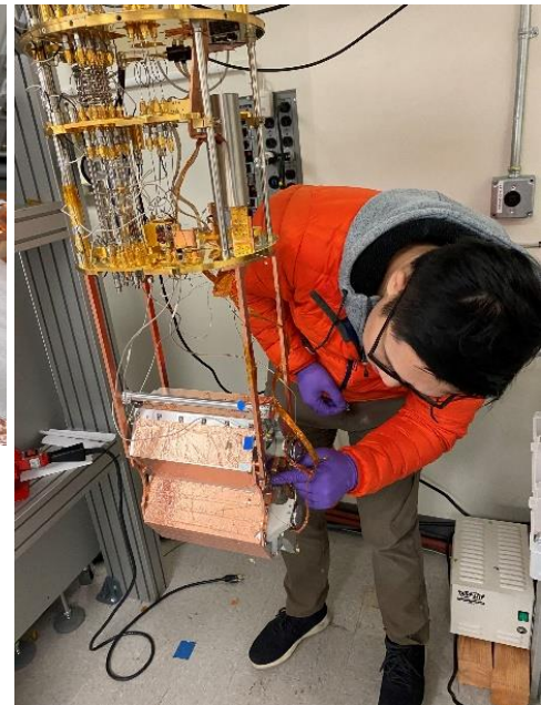
Postdoc Nick Du mounting scale length prototypes in dilution refrigerator
