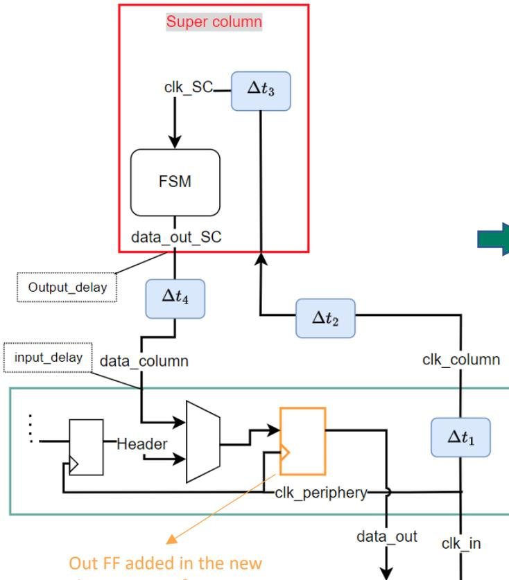
Out FF added in the new chip to satisfy output timing constraints
