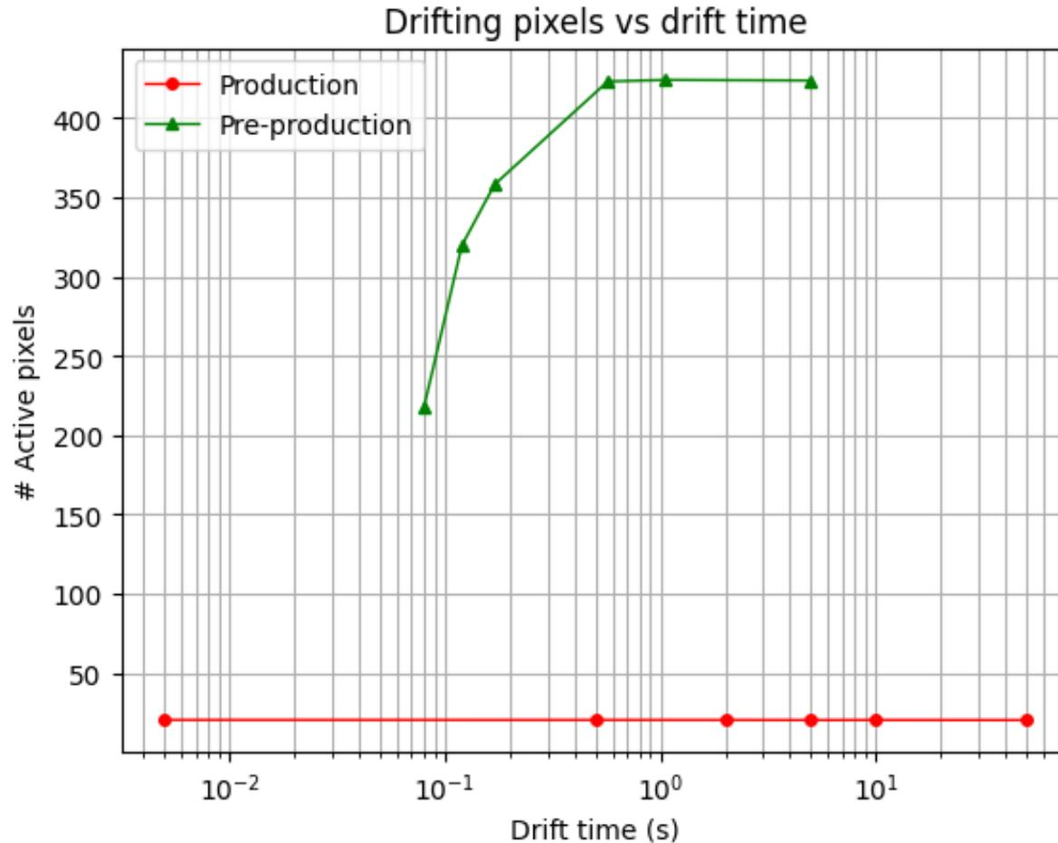
Analogue memories **leakage** could modify the memory value:
