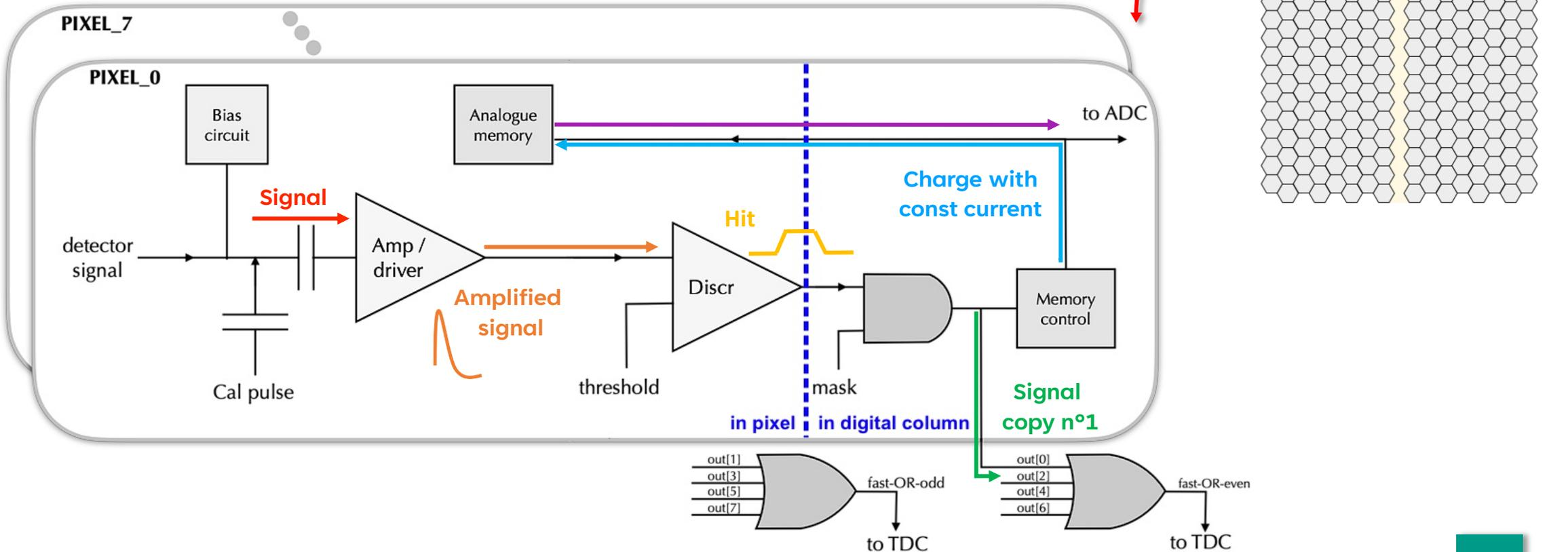
**Analogue memories: capacitors inside each pixel charged with constant current during ToT**
