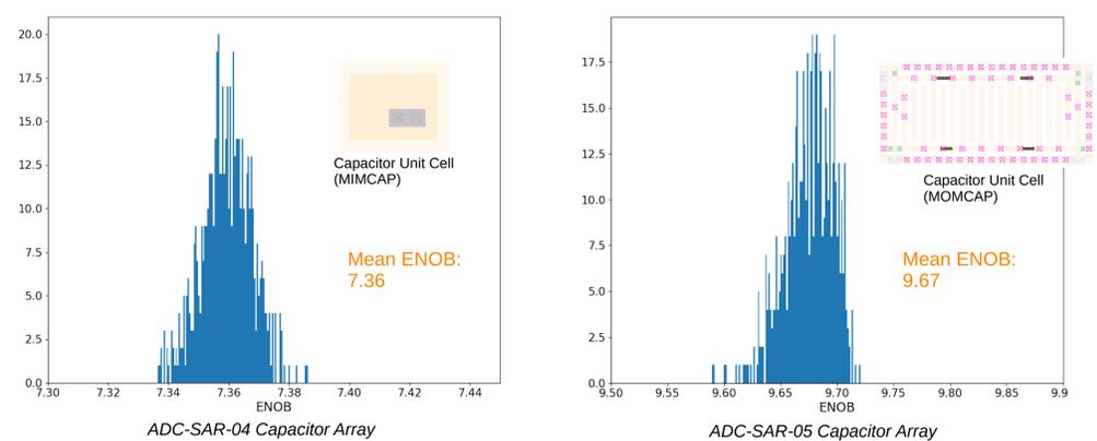
**New unit cell** (and layout) of the capacitor array **improves the mismatch** contribution to the ENOB by ~2 bits. Figures show a Monte-Carlo simulation for the random mismatch (given by the foundry) including static mismatch due to parasitic coupling (extracted from layout).
