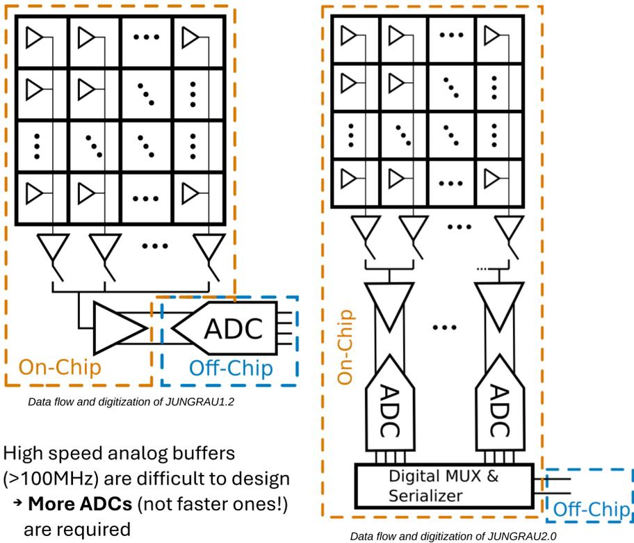
High speed analog buffers (>100MHz) are difficult to design
