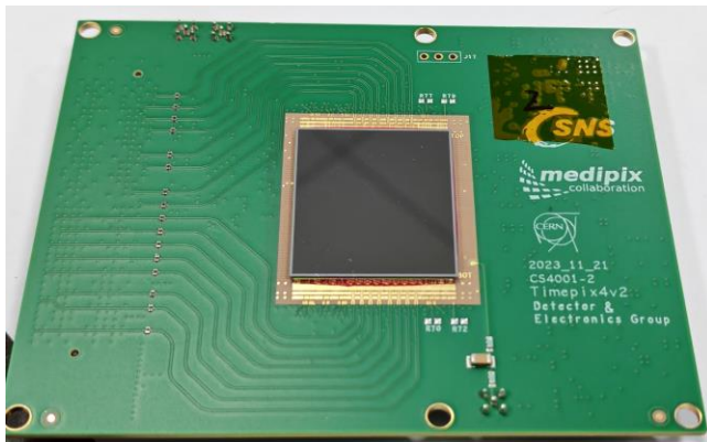
Chip Board with TPX4 300um Si
