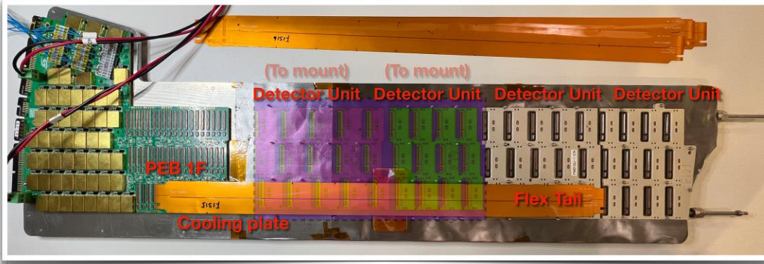
HV, LV, Cooling plate prototype
