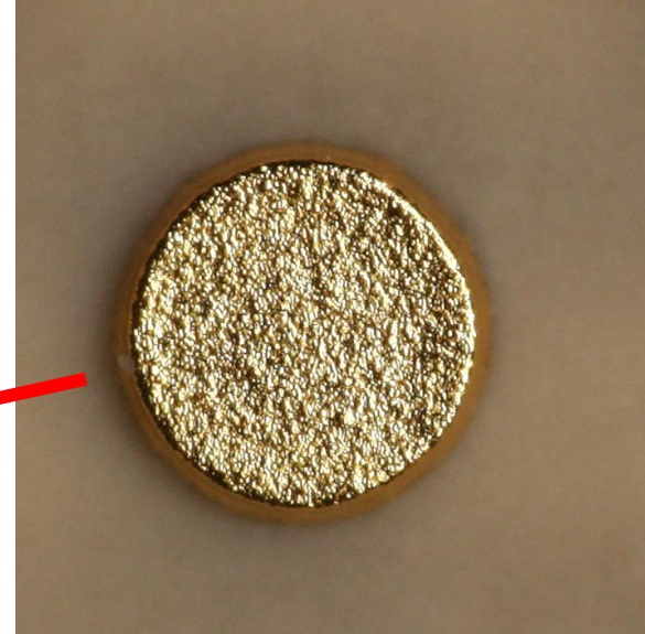
PCB BGA pad before glue
