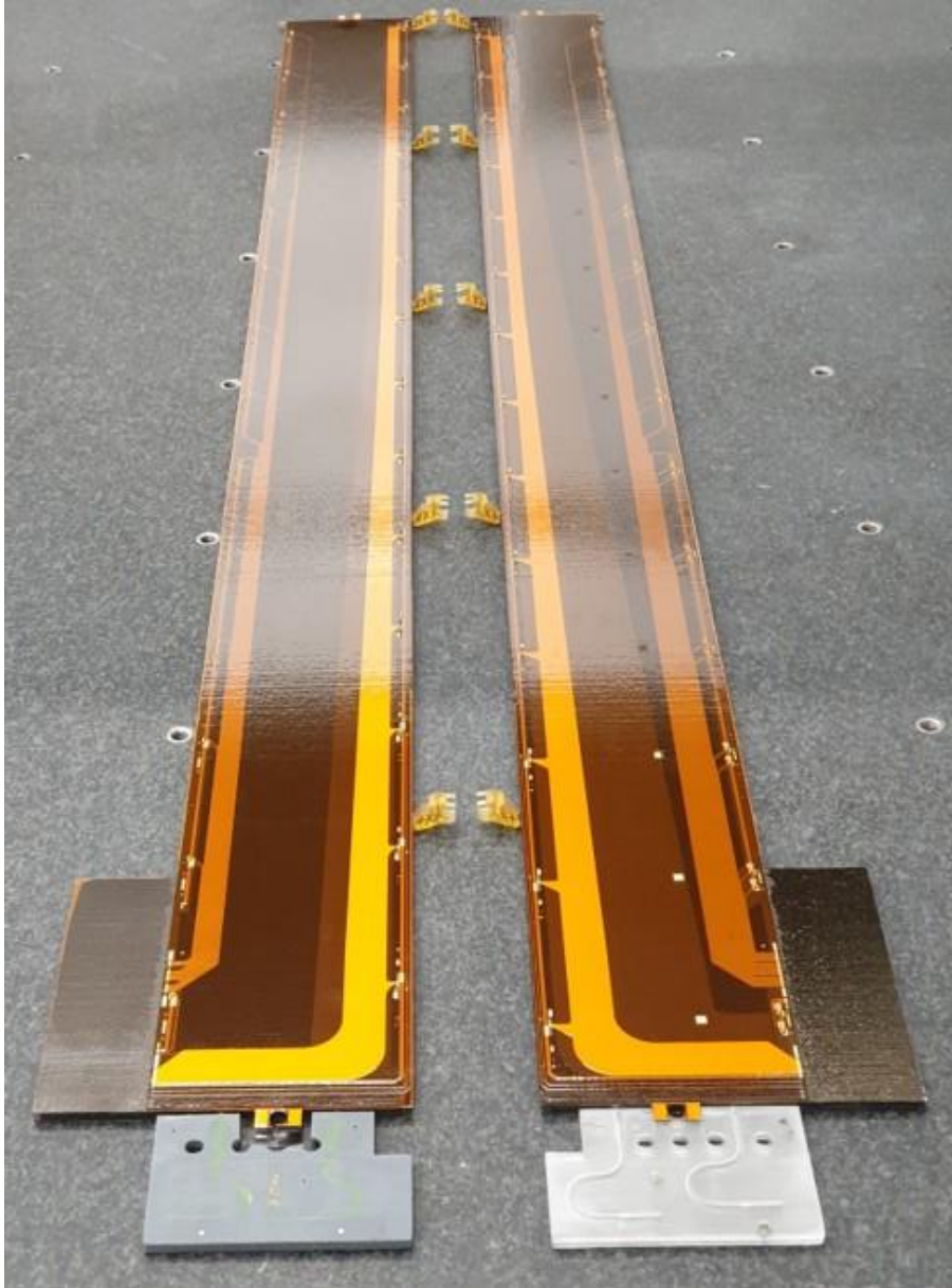
2 Barrel tapes integrated into carbon fibre cores
