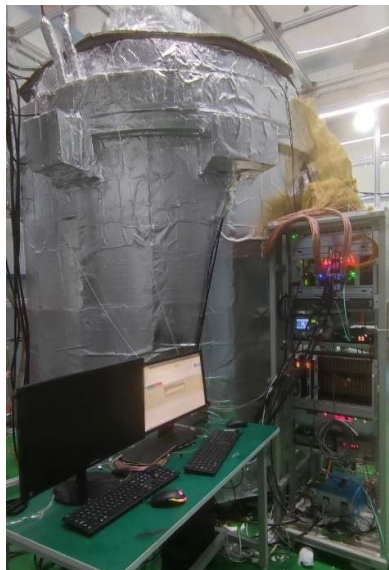
Fig. 4 Photo of 1:1 detector prototype and the readout system with WR
