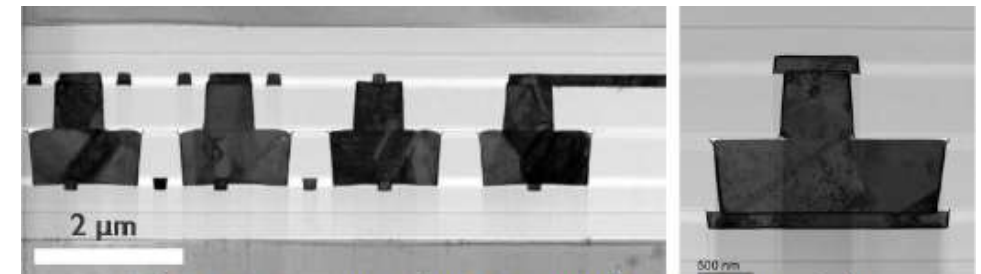
Fig. 11. TEM 540 nm pad on 1260 nm pad array at 1.8 μm pitch.
