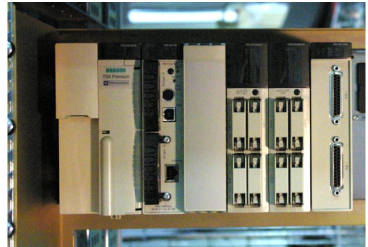
PLC modules for ArDM (Schneider Electric Modicon Premium)
