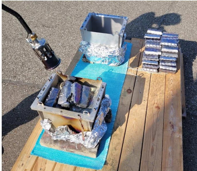
Lead buffer casting
