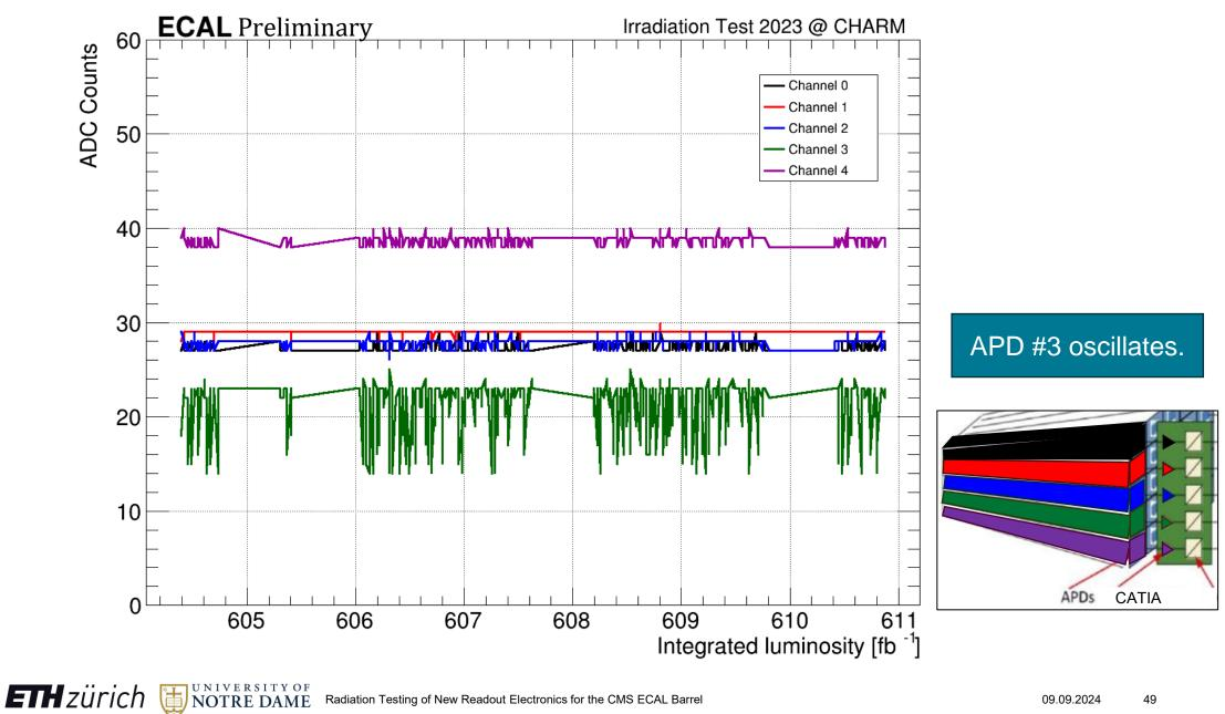
Radiation Testing of New Readout Electronics for the CMS ECAL Barrel
