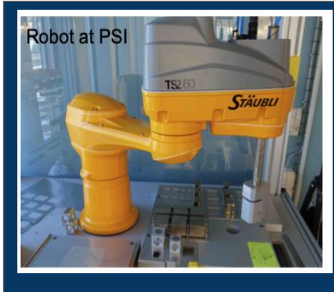
Module assembly using robotic arm at PSI
