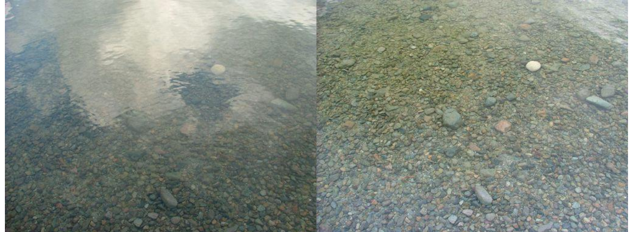
Photography: elimination of reflections on the water surface, without (left) and with (right) polarizer
