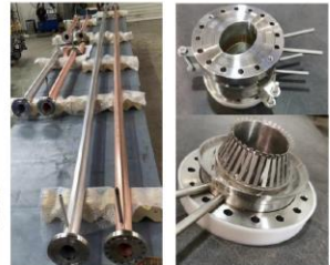
Vacuum pipes and RF shielding bellows
