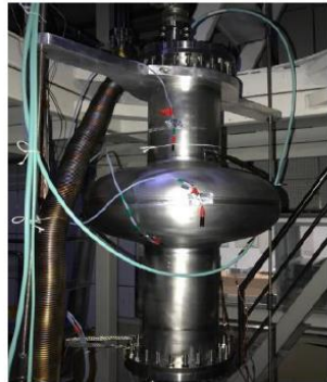
Vertical test of 650MHz 1-cell cavity
