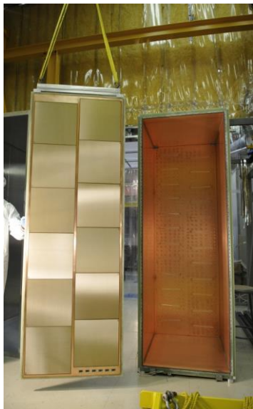
T2K TPC ,J.Beucher 1.8m x 0.8m plane With 12 detectors
