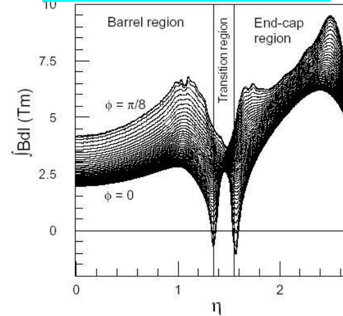
Field integral inhomogeneous in the tracking volume
