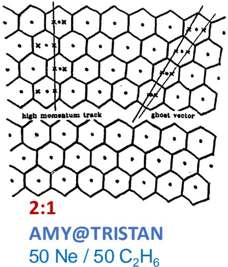
**Closed cells** limit the very long tails in the drift time distribution, make the t-to-d (x-t) relations more uniform and less dependent from the track angle
