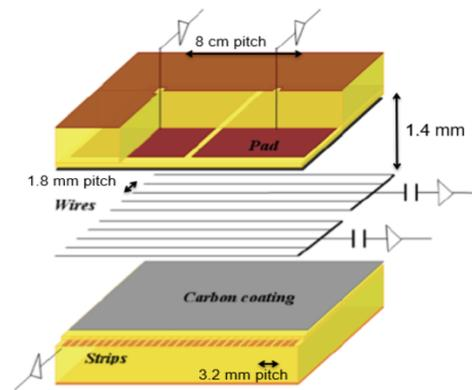
sTGC → strips with 3.2mm pitch, increased resolution to operate at high background rate reducing the muon fake rate
