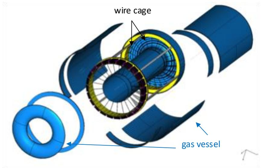
Inner cylinder and Outer cylinder connected with 48 Spokes (24 per Each side) forming 24 azimuthal sectors.
