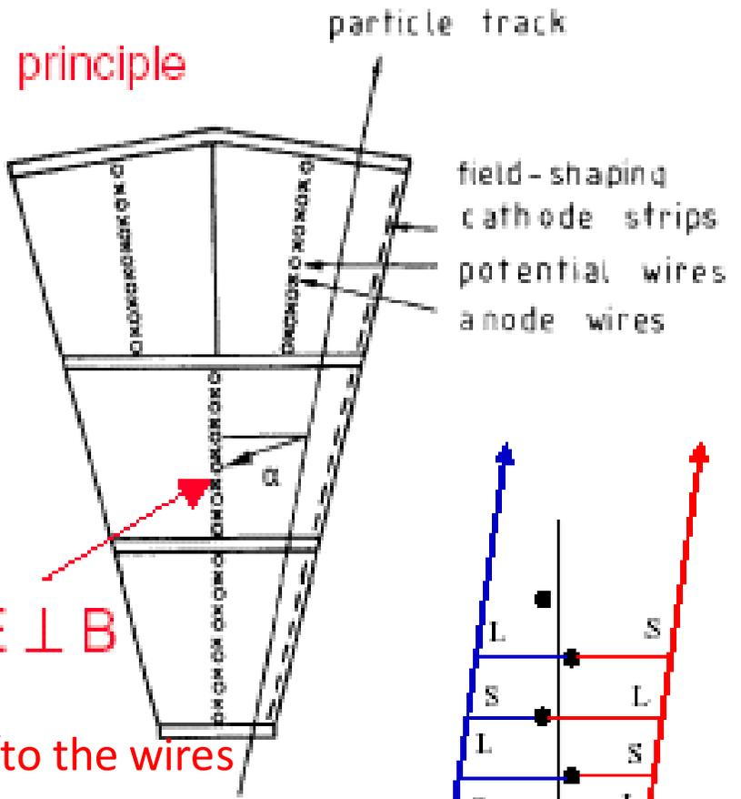
$\varnothing=3.7\text{m}$ ,  $L=4\text{m}$ , 24 sectors with 159 sense wires ( $\pm 100\ \mu\text{m}$  staggered).  $3\ \text{cm} < l_{\text{drift}} < 25\ \text{cm}$
