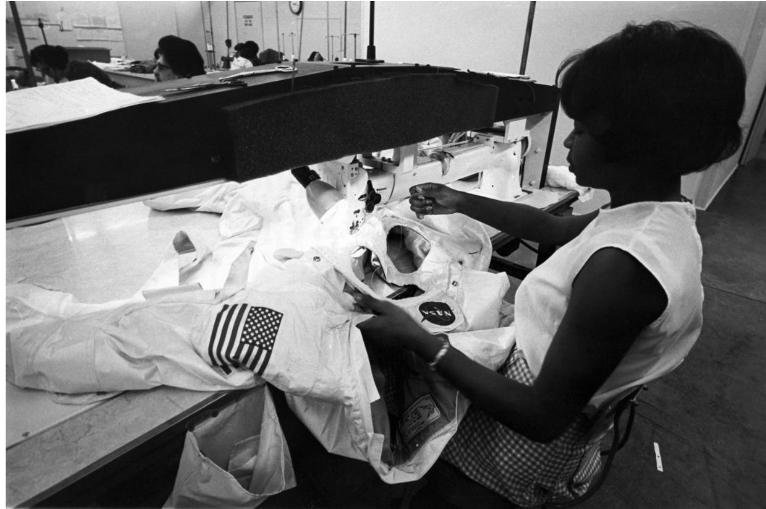
Hazel Fellow, machine sewing an Apollo spacesuit at ILC. (Smithsonian National Air and Space Museum)
