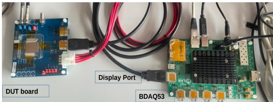
TJMP2 setup DAQ inherited from RD53 collaboration
