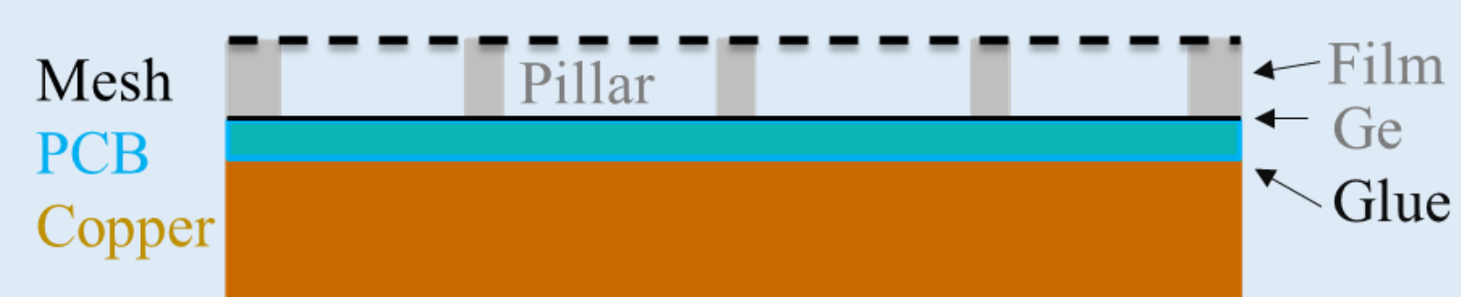
Fig 2. Schematic diagram of structure and corresponding materials of thermal-bonding Micromegas.
