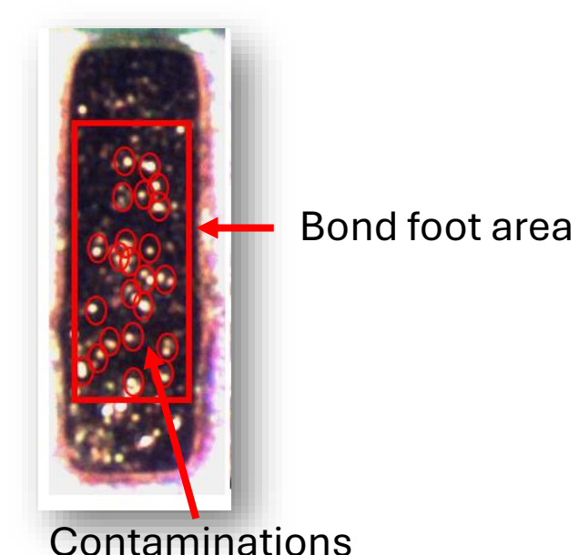
Opened glue joint in a PS-Front-End Hybrid
