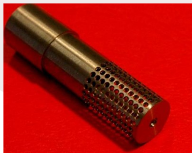
IRENA (Ionization by Radial Electron Neat Adaptation) prototype based on EBG (Nitschke, LBL 1985).
