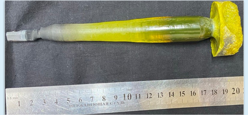
YAG:1%Ce,0.75%Ca,0.25%Mg single crystal
